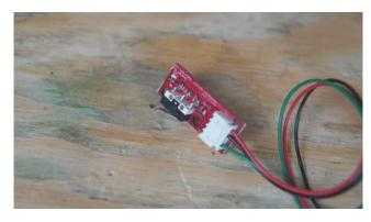
In this guide, we'll be using a 3 wire style limit switch, mounted to a printed circuit board to make installing it on your machine easier.
