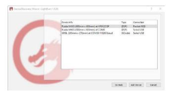
In this example, I have two lasers connected to my computer — a Ruida DSP controller on COM3 and a GRBL controller on COM30. Select your laser and click  $\,$  Add  $\,$  Device .
