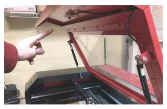
Camera installed in a laser
