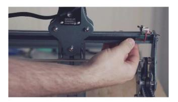
You can use 2020 extrusion covers cut to size to protect and hide the wires inside the grooves of the extrusion frame, and zip-tie the limit switch cable for the gantry to the pre-existing cable to the diode head itself.
